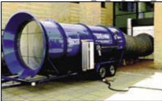
Fig 18: Large fan for testing industrial buildings
