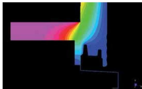
Figure 22: Typical heat flow pattern through insulated metal junction determined by finite element analysis.
