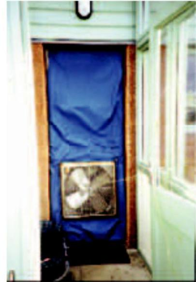
Fig 31: Typical 'Blower Door' for testing domestic buildings
