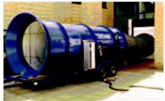
Fig 32: Large fan for testing industrial buildings
