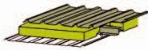
Fig 6: Roof with profiles and zed spacers at right angles
