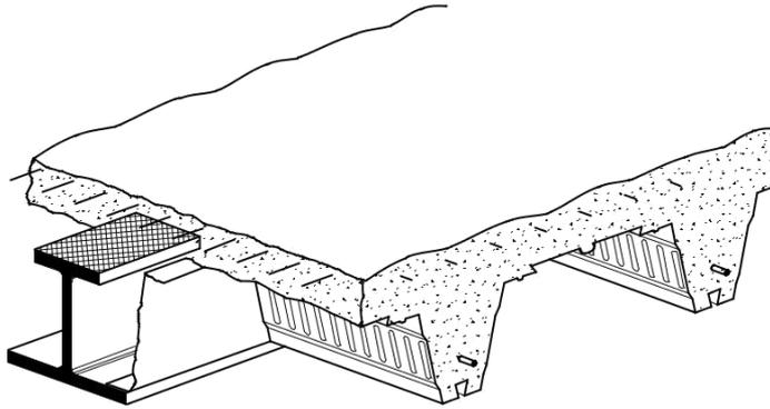
**Figure 7.2** ASB with deep decking (composite beam)
