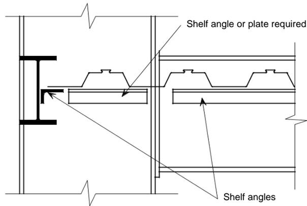
**Figure 4.7** Decking support details at a column web
