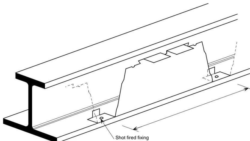
**Figure 7.17** Fixing of end diaphragms at ASB
