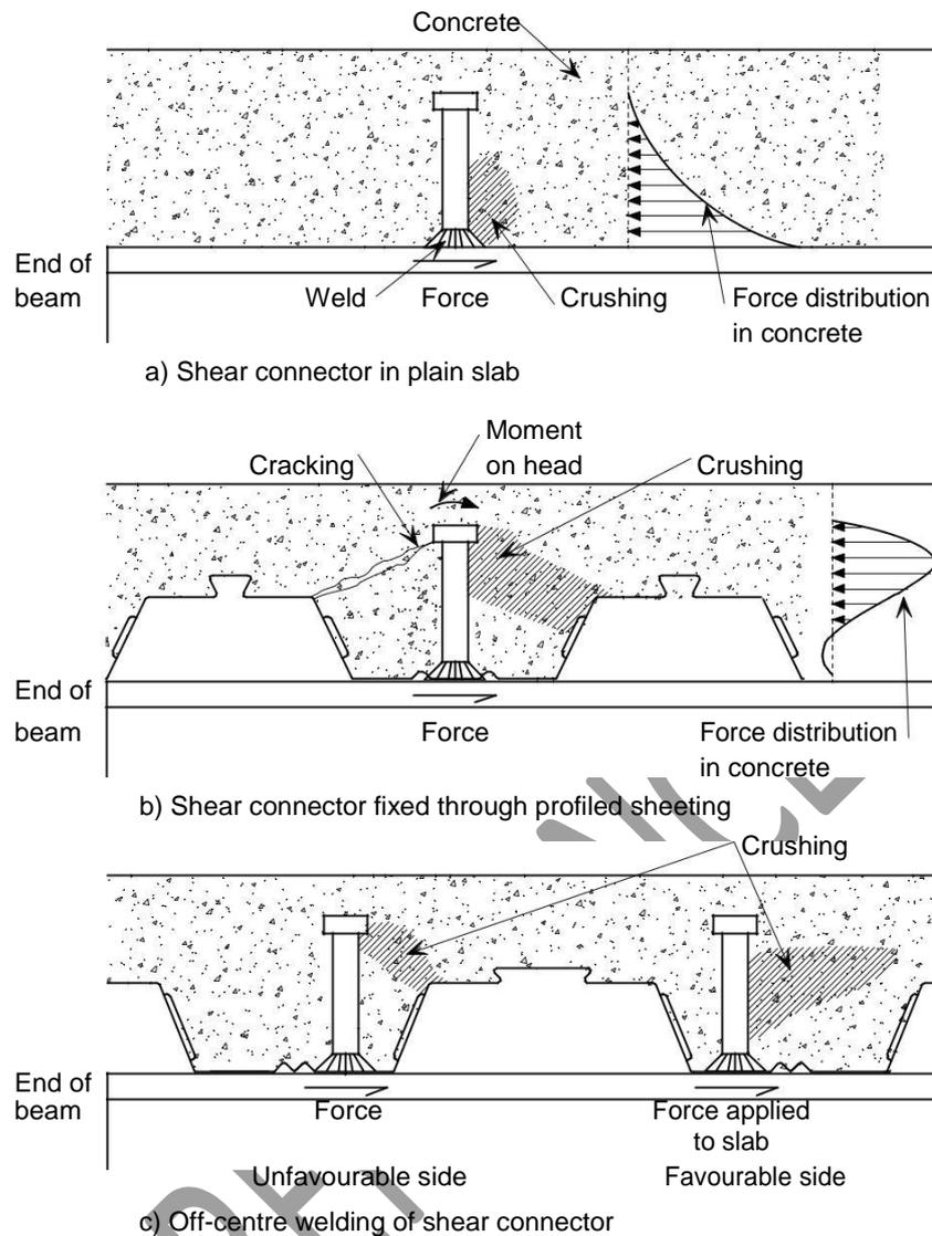
**Figure 5.5** Shear connector forces in composite slabs
