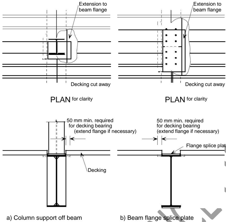
**Figure 4.8** Decking details where a column is supported off a beam and where a beam flange splice plate occurs
