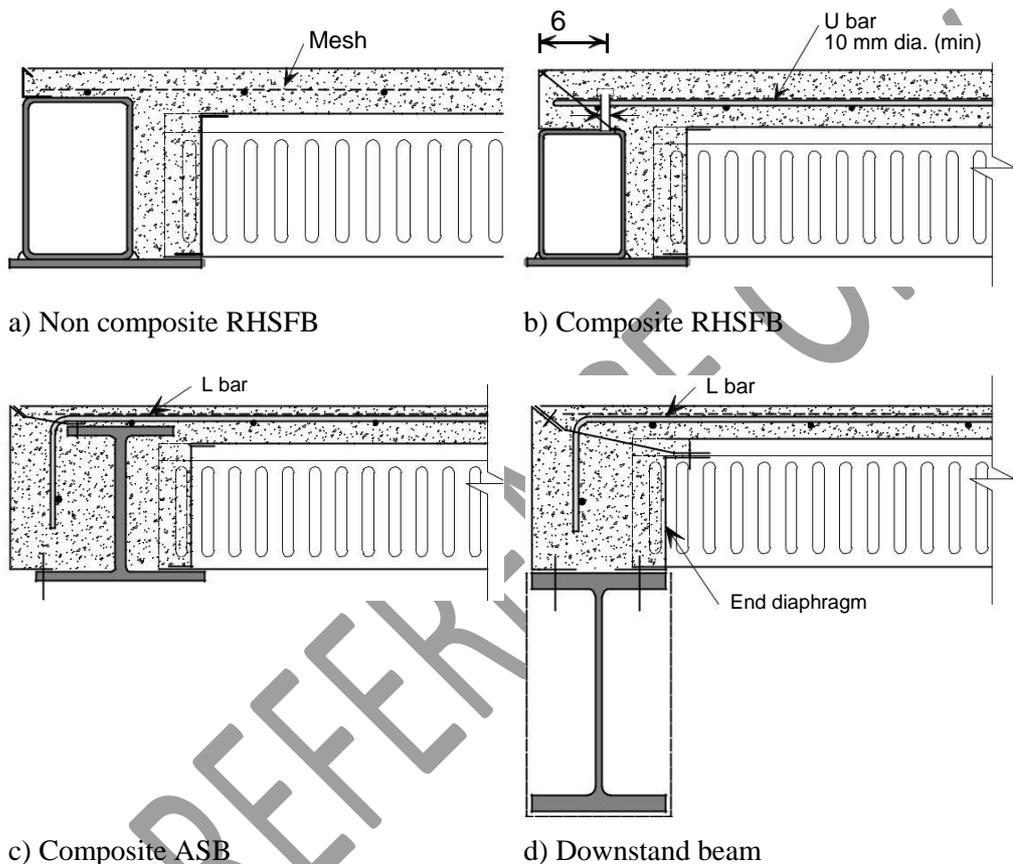
**Figure 7.14** Typical edge beams.
