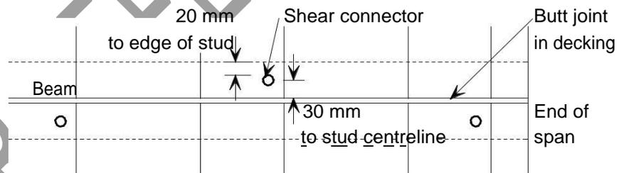
d) Butt joint in decking (correct positioning of single stud per trough)
