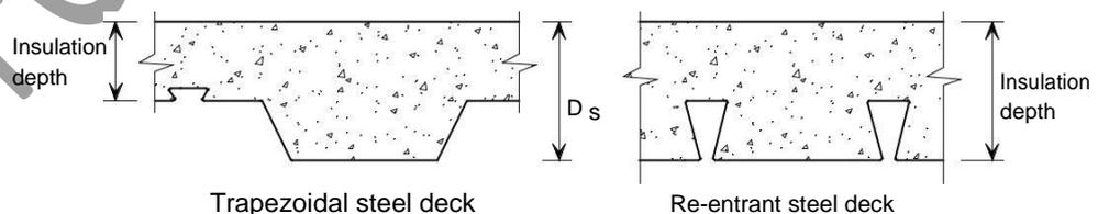
**Figure 4.10** Minimum insulation depth measurement
