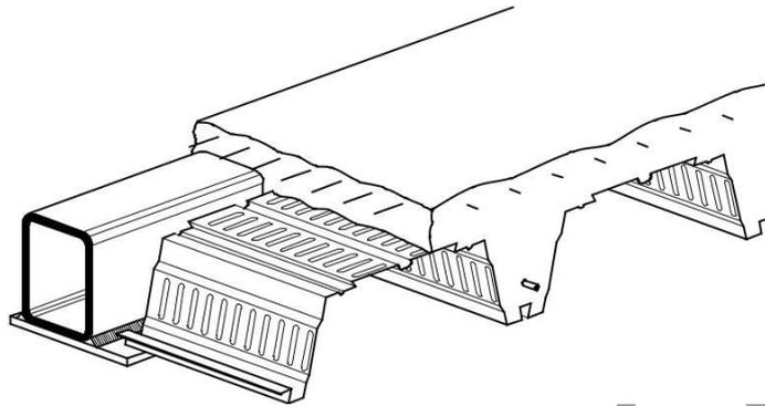
**Figure 7.3** RHSFB with deep decking (non-composite beam)
