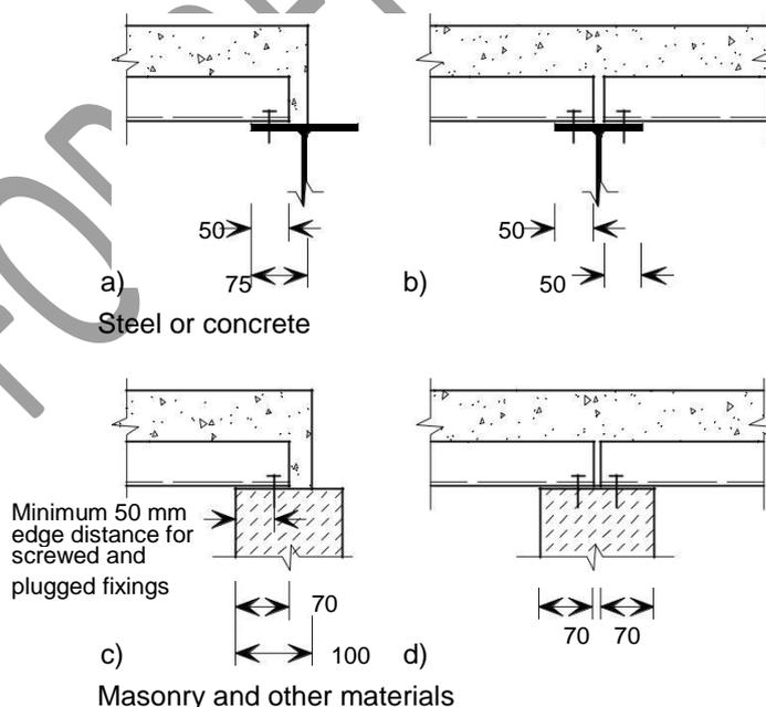
**Figure 4.5** Minimum bearing lengths for permanent supports
