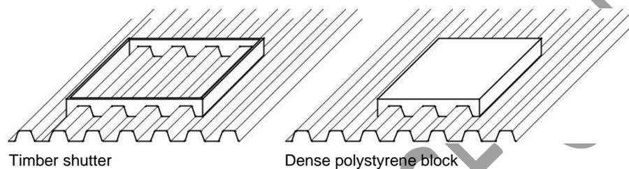
**Figure 4.11** Typical examples of boxing out openings
