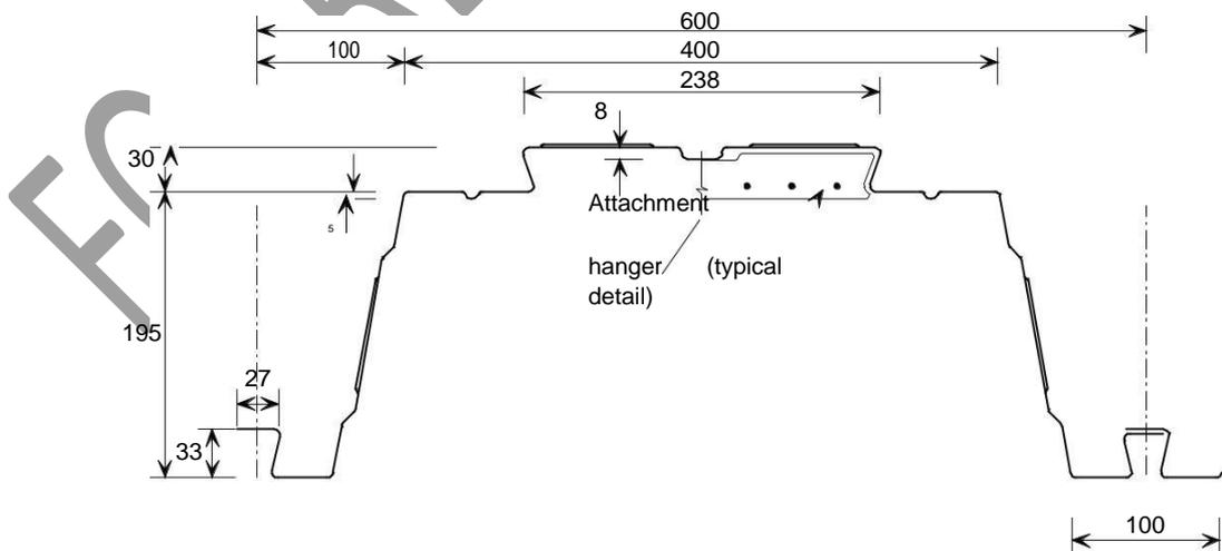
**Figure 7.4** Cross-section of *ComFlor 225* deep decking profile, showing a typical service attachment detail.
