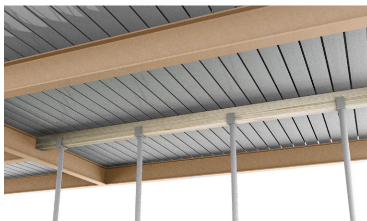
Figure 4.18 Temporary support using 'Acrow' props
