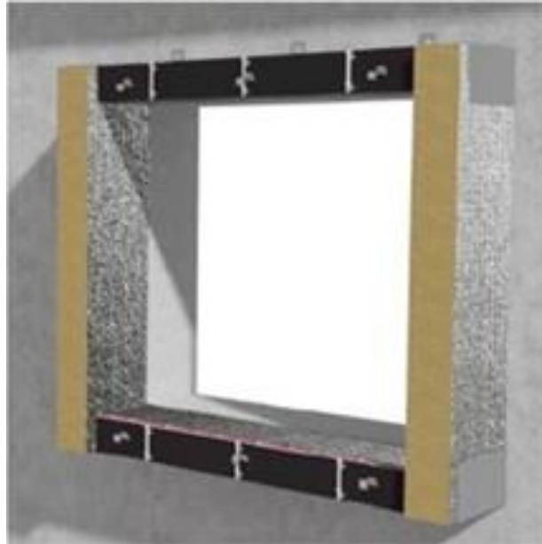
Image shows closed state vertical cavity barriers on the jamb of an opening and horizontal open state on the head and cill.
