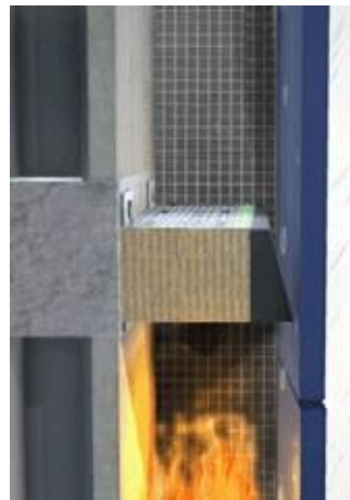
Intumescent strip on the face of the horizontal open state cavity barrier starts to react and expand due to the heat created by the fire
