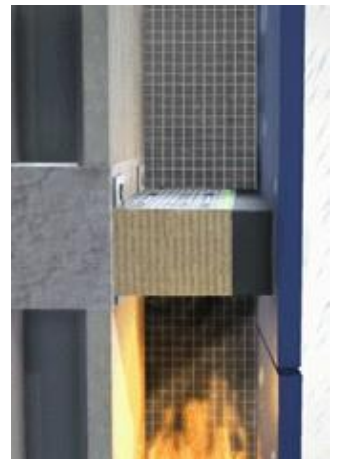
Cavity is closed and sealed
