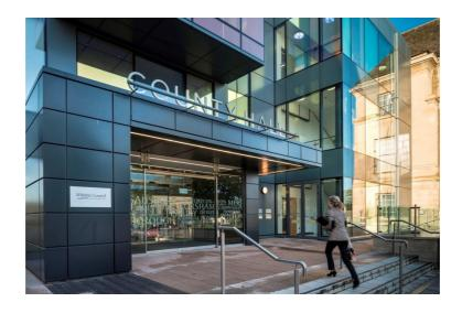
Architectural Profiles' Slimwall CPS aluminium rainscreen system was specified for the redevelopment of Trowbridge County Hall to provide a retrofit building envelope which could achieve a 40 per cent reduction in carbon emissions. The building has achieved a BREEAM 'Excellent' rating. Image courtesy of Architectural Profiles
