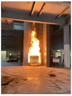
A rainscreen and facade manufacturer is leading the way in safety after its latest product became one of the first in the UK to be tested against the latest BS 8414-2 standard – despite the upheaval caused by Covid-19.
