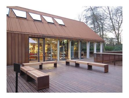
The walls are made from wood and glass, to reflect the wood and water found in the estate. The land itself is reflected in the choice of Cor-Ten steel for the roof and some outer walls. This is a distinctive looking material that has been used to great effect in a number of buildings and sculptures, including Kew Gardens and the Angel of the North.
