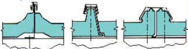
Fig. 12 SIDE LAP JOINTS - SLOPES GREATER THAN 1°
