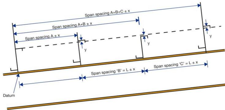
*Figure 2 Limits on span position*
