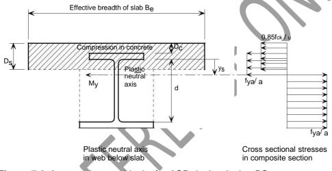
Figure 7.6 Assumed stress blocks for ASB design (using BS EN 1994-1-1 notation)
