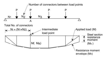
Figure 5.11 Shear connector distribution for beams subject to point loading
