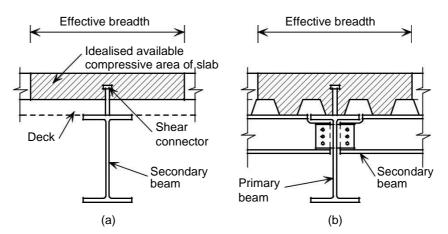
Figure 5.4 Composite beams incorporating composite slabs. (a) Deck perpendicular to secondary beam. (b) Deck parallel to primary beam
