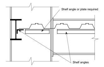
Figure 4.7 Decking support details at a column web
