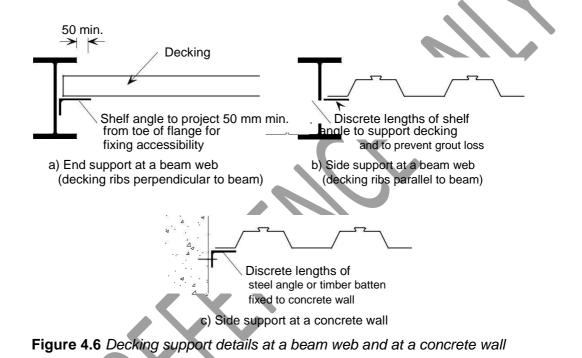
Support is also required when the decking interfaces with a concrete wall. This may be provided by attaching a steel angle, flashing, or timber batten to the wall, preferably by using cast-in fixings (Figure 4.6(c)). Provision may need to be made to achieve reinforcement continuity between the wall and slab.
