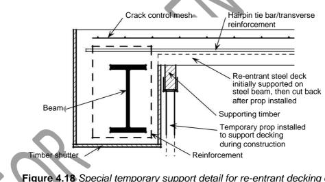
Figure 4.18 Special temporary support detail for re-entrant decking on a concrete-encased beam
