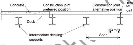
Figure 6.2 Recommended positions for construction joints in the concrete slab
