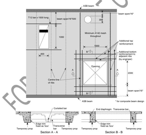
Figure 7.12 Details of small and medium size openings in the slab.
