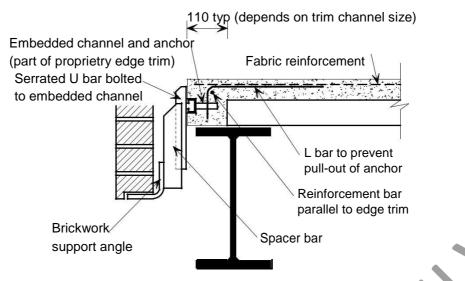
Figure 4.20 Typical steel brickwork support
