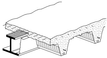
Figure 7.2 ASB with deep decking (composite beam)
