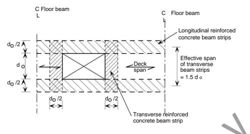
Figure 4.13 Load paths and beam strips around medium to large openings
