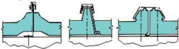
Fig. 12 SIDE LAP JOINTS - SLOPES GREATER THAN 1°
