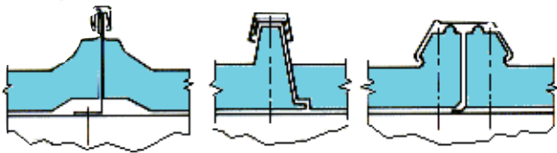
Fig. 12 SIDE LAP JOINTS - SLOPES GREATER THAN 1°
