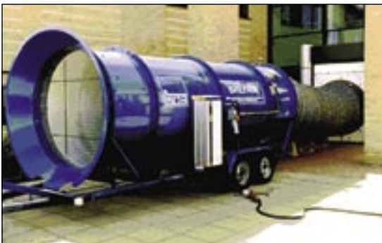
Fig 18: Large fan for testing industrial buildings
